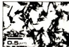
Metal particles with virtually ideal size, shape and ferromagnetic properties.
